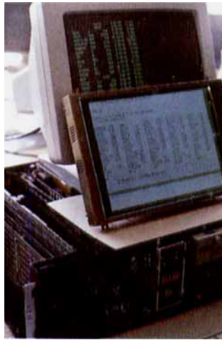
Figure 7. 400 line multiplexed black–white supertwist LCD in front of a cathode ray tube terminal.
